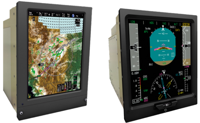
Figure 3. Multifunction display showing different applications (Source: ScioTeq)
